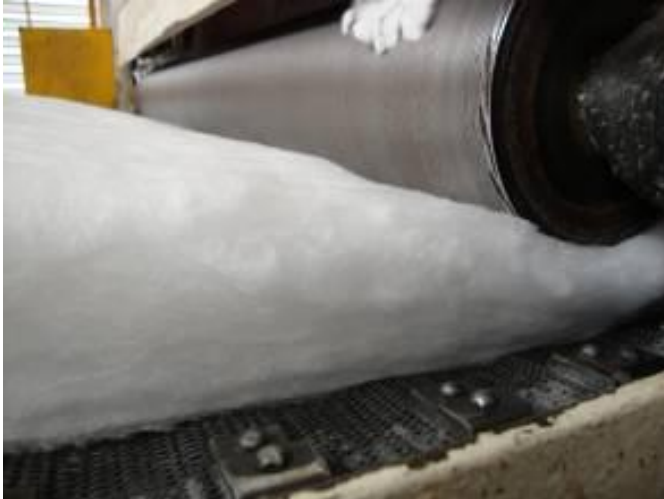
Fibre fleece before needling
